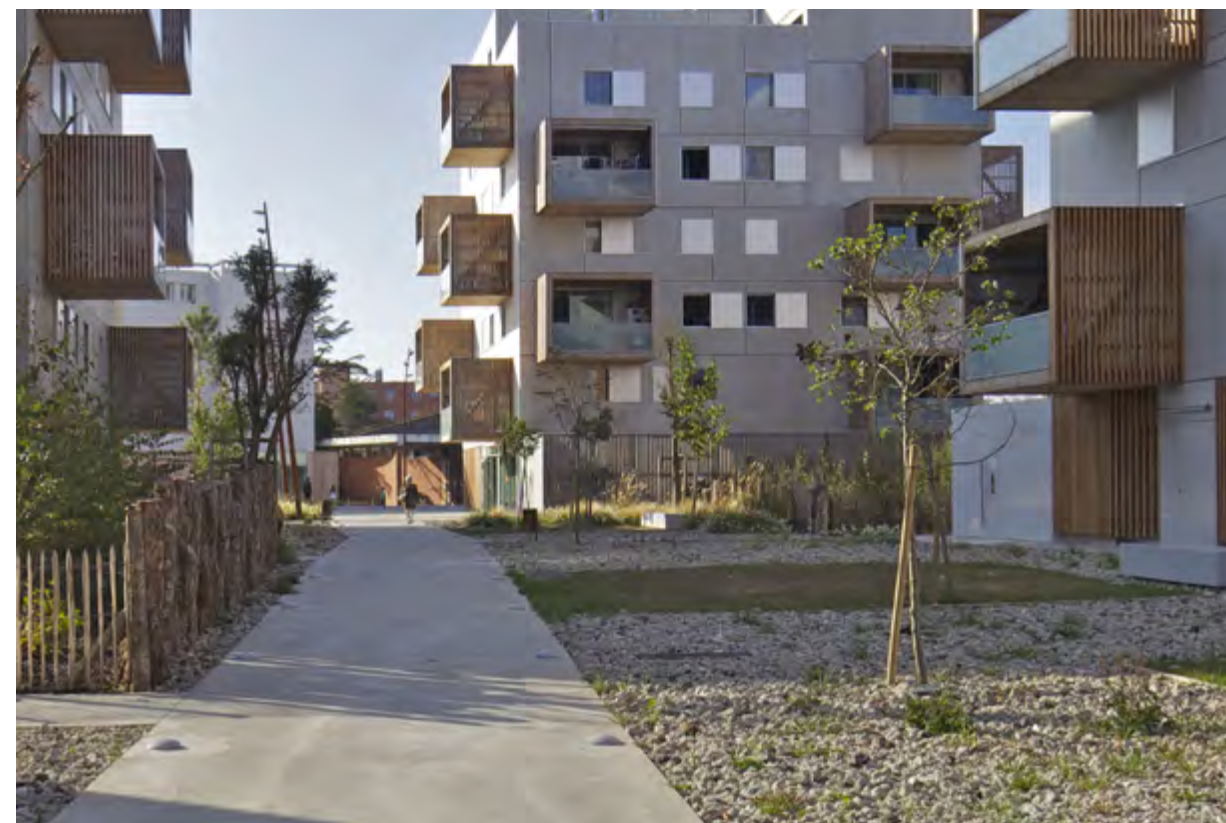
Crushed concrete used as mulch layer ↑
