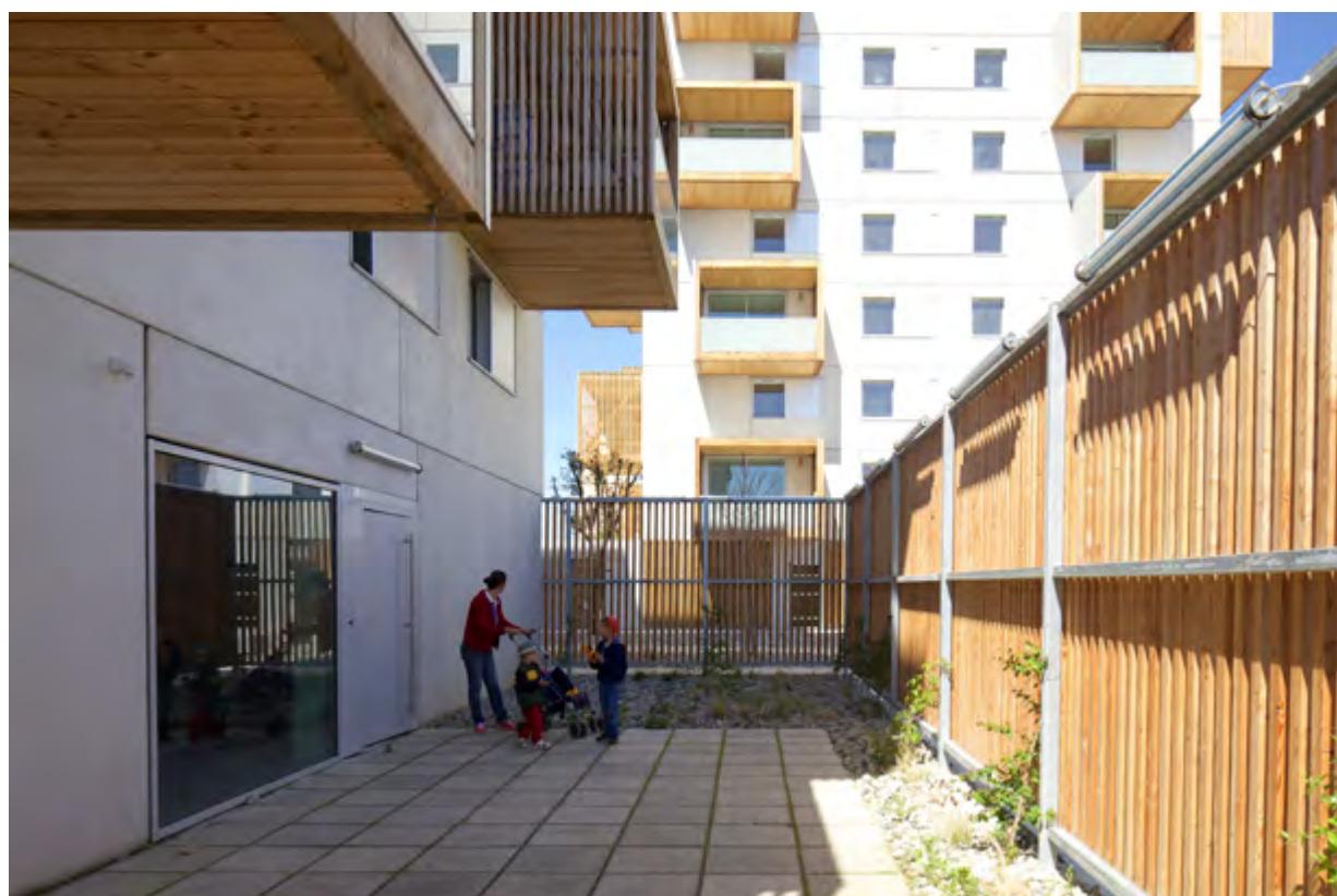
↓ Collective small courtyards in concrete slabs reclaimed from the former shopping centre
